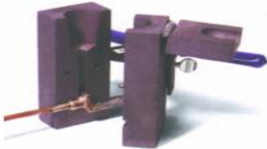
FIGURE 6-48 EXOTHERMIC WELDING MOLD (LEFT) AND PROCESS (RIGHT)
